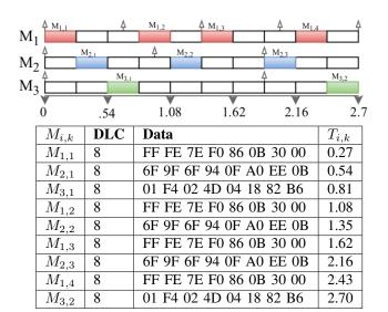
at high frequency to override normal vehicle operations. These malicious messages were constructed by spoofing legitimate messages transmitting on the bus. We identified message IDs such as wheel speed and backup light while observing the
